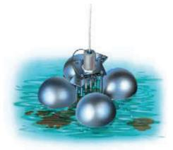
If, for example, oil flows onto a still water surface following a leak, exact setting of the rod electrode will ensure that an oil layer of only approx. 5 to 10 mm thickness is sufficient to interrupt the control current flowing via the rod electrode and activate an alarm.
